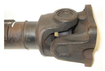
The factory original front driveshafts found on Jeep Liberty 3.7L models from 2008-2012 has a non-replaceable staked-in style u-joint. With the Rockford Driveline parts below you are able to cut the Original assembly apart 1/4" below the friction weld and replace the Weld Yoke, Flange Yoke & U-Joint with a servicable 1310 system.
